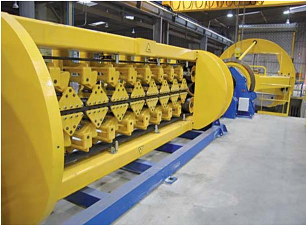
**Drum tester 4000 mm for Milliken conductors up to 3000 mm<sup>2</sup> from C.M. Caballé.**
